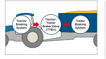
Fig.2 Role of the tractor-trailer brake valve (TTBV)
