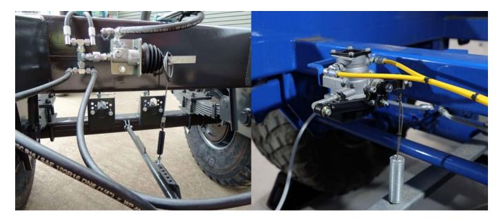
Fig.24 Hydraulic (above) and Pneumatic (right) trailer Load Sensing Valves
