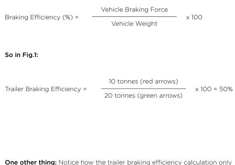
**One other thing:** Notice how the trailer braking efficiency calculation only uses the weight carried by the vehicle's wheels? (e.g. 20 tonnes in Fig.1) But many trailers also transfer a vertical load onto the tractor via the drawbar. This increases the tractor's weight and adds to its own braking load. So when towing a trailer, the tractor's brakes have to work harder than when travelling solo, even if the trailer's brakes are working perfectly!
