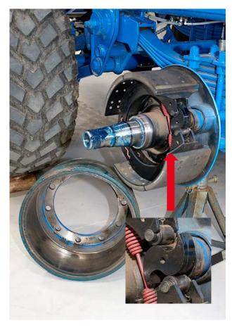
Fig.14 Example Commercial 'High-Speed' brake and drum- Note 'S'-type operating cam (arrowed & inset)
