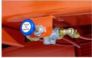
Fig.10 Shunt valve fitted to an air-braked trailer
