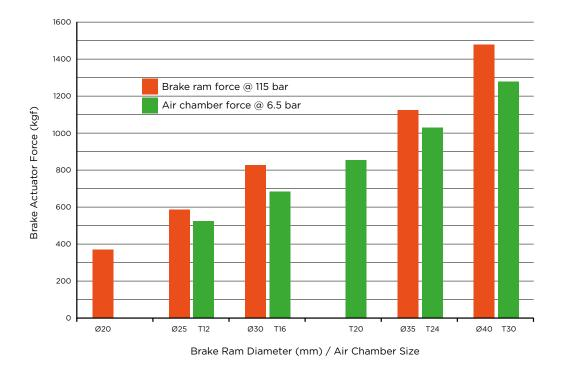
Fig.16 Effect of brake ram or air chamber size on brake actuation force
