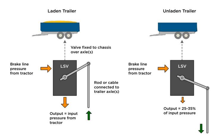
Fig.23 Load Sensing Valve (LSV) operation
